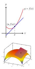
In calculus of one variable, the derivative f'(a) defines a *tangent line* to the graph of *f* at (a, f(a)) by the equation
