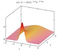
For each t we get a "snapshot" of the distribution of heat–at first heat concentrates near x = 0, but then diffuses and cools as time moves forward
